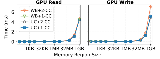
Figure 4. GPU READ and WRITE performance on Spark under different cache and CC policies. 1-CC denotes one-way coherence, and 2-CC denotes two-way coherence.
